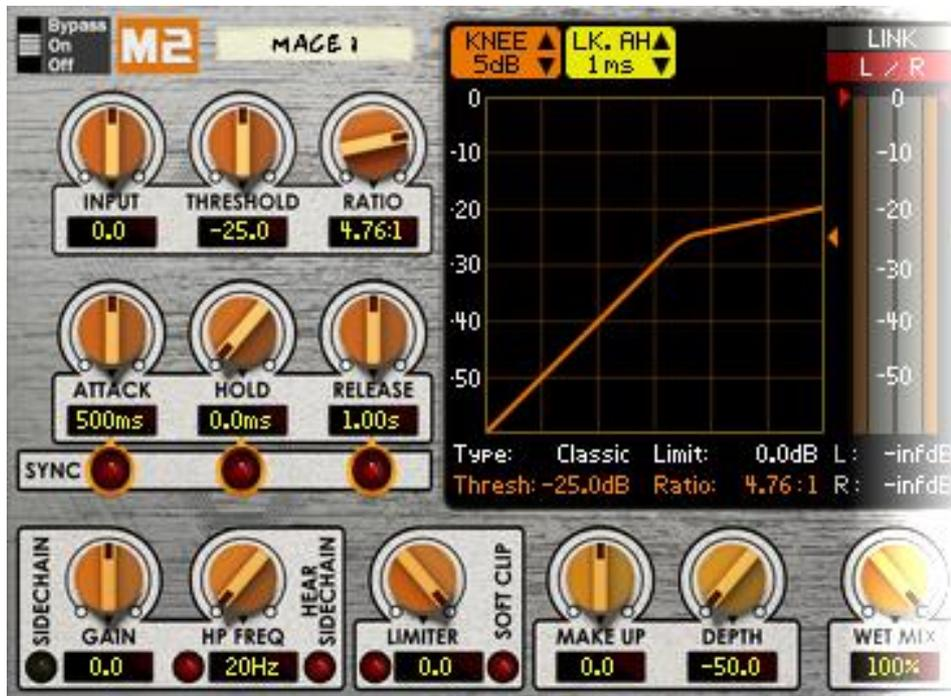
The Mace has 2 sets of controls for compression, for each channel. The left side controls the compression for the left signal (in unlinked mode) or the mid signal (in mid/side mode). The right controls in turn control the compression if the right signal (in unlinked mode) or the side signal (in mid/side mode). The only exception is in linked mode, where only the left controls will be used to affect both left and right channels together in tandem.
